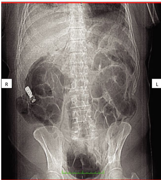
FIG. 5—Posttest computed tomography image of Torso 2 with the shot 2Q1 extended range electronic projectile inside the abdomen (anterior view).
