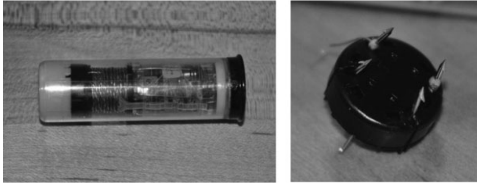
FIG. 2—Left: Representative extended range electronic projectile inside a 12-gauge cartridge. Right: Close-up of the detachable tip section (right).
